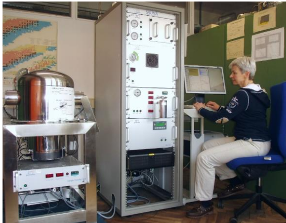
SAUNA - Lab \beta - \gamma coincidence detection system
