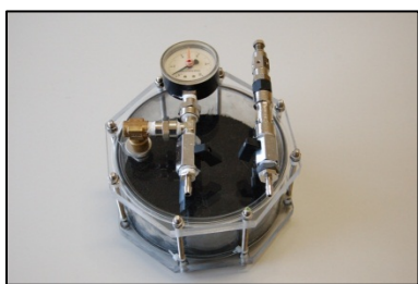
Plexiglas container containing the exposed charcoal (left) and its positioning in the shield of the germanium detector (right)
