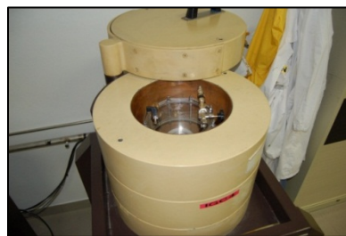
Plexiglas container containing the exposed charcoal (left) and its positioning in the shield of the germanium detector (right)
