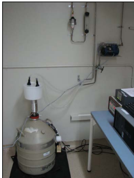
Figure 5.2. ANSTO prototype high-resolution stack monitor.
