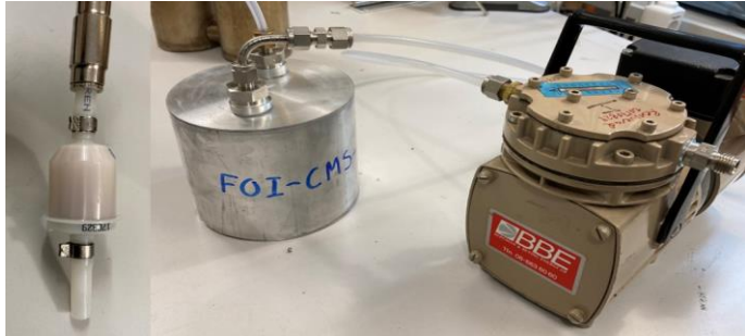
Sampling equipment (CMS trap, filter, and pump).
