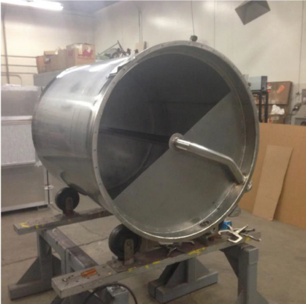
Figure 9 - Inspection of Carbon Column Post Testing
