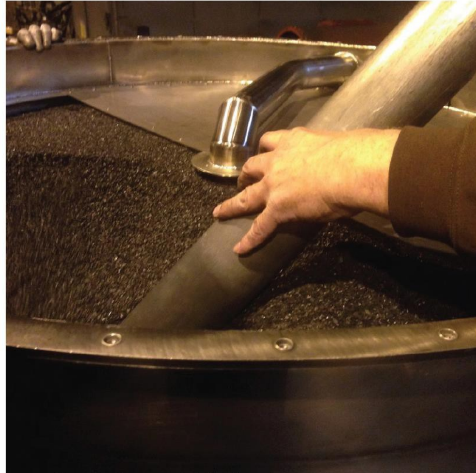
Figure 8 - Removal of Carbon from Carbon Column post testing
