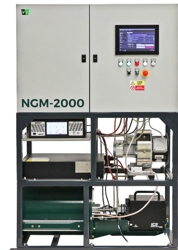
VF Nuclear High-purity germanium (HPGe) detector installed in SHINE
